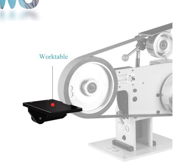
The worktable is suitable for each grinding wheel. It can be disassembled and easily polished for various shapes. Compared with the handheld, it can provide a more stable operating environment and support greater cutting force.
